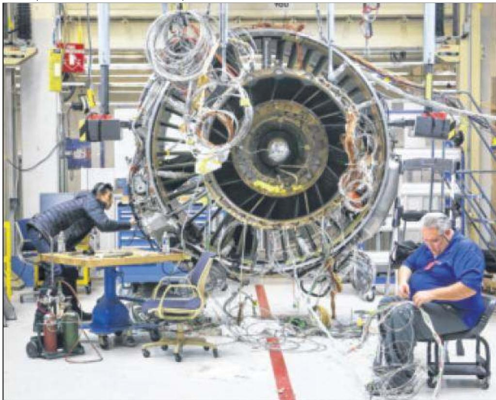
The LEAP commercial jet test engine, which is being worked on in Evendale, is a product of a joint venture between GE and French manufacturer Snecma. The engine will be more fuel efficient and contain advanced materials. **STAFF / 2014**
